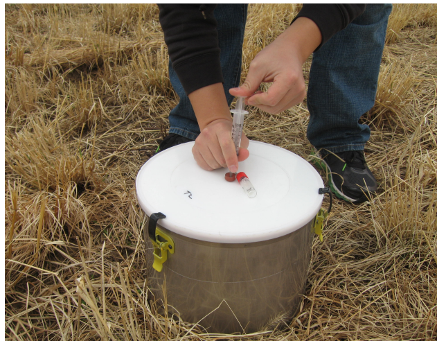
Figure 18. Chamber mixing and headspace sampling.
