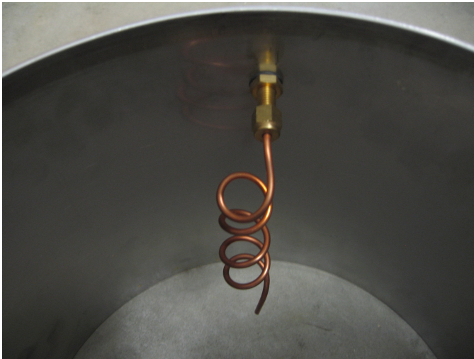
Figure 12. Inside view of a chamber vent.
