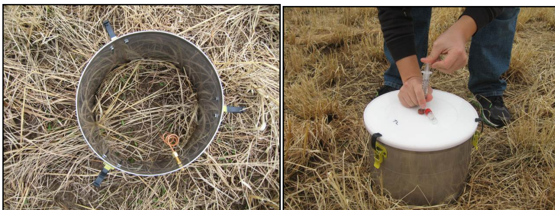
Figure 1. Static chamber as deployed in the field prior to (left) and during (right) gas sampling.
