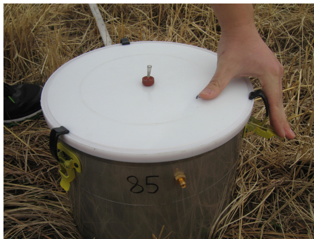
Figure 17. Chamber lid deployment using needle vent.
