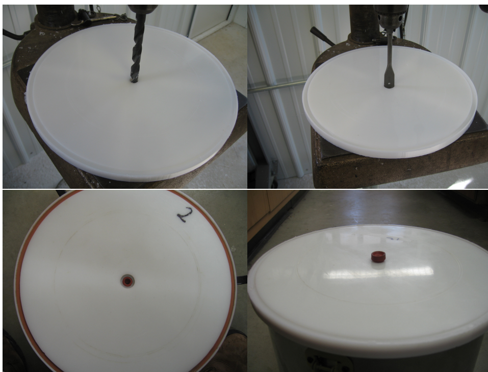
Figure 10. Installation of sampling septum.
