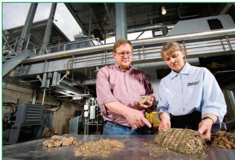
Figure 2. At the University of Minnesota-Morris Biomass Gasification Facility, researchers evaluate potential biomass feedstocks, including pressed corn stover.
