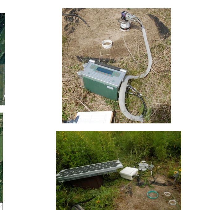
Figure 4. The measurements of R_s and R_p . We used LI-8100 or LI-6400 to measure in situ SR with soil temperature and soil moisture.
