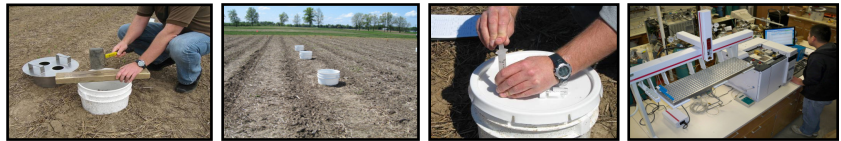
Static chamber deployment and sampling in field and automated sample analysis in laboratory.
