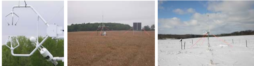
Fig 1. The Eddy covariance instruments at GLBRC scale-up plot fields
