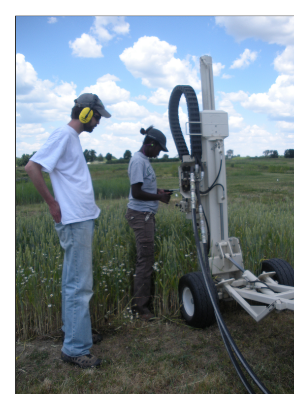
Field Sampling: A geoprobe was used to extract soil cores to a depth of 1 m.
