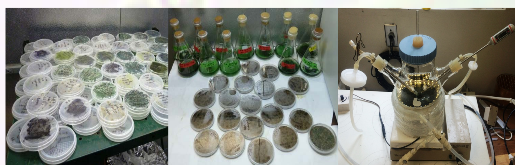
Figure 2. Different cyanobacterial cultivation systems. From left to right are agar plates, flasks, soil microcosms, and photo-bioreactors.
