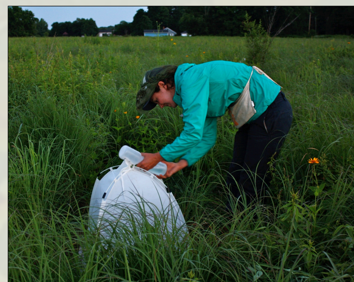
Figure 2. Placing collection jar half-filled with 2% soap solution at top of emergence trap in mature wildflower planting.
